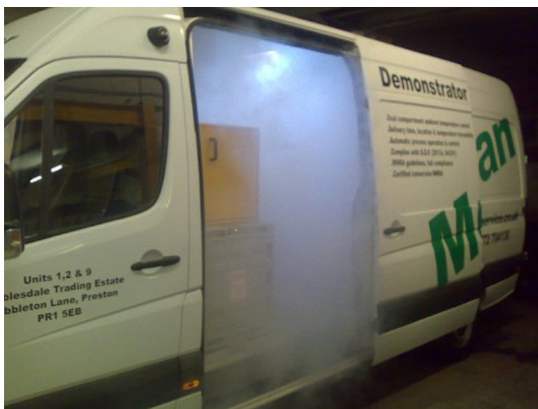
Cargo area being smoke tested to ensure integrity of the internal lining & door seals
